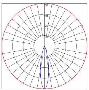
Maximum Candela = 753 Located At Horizontal Angle = 0, Vertical Angle = 0 # 1 - Vertical Plane Through Horizontal Angles (0 - 180) (Through Max. Cd.) # 2 - Horizontal Cone Through Vertical Angle (0) (Through Max. Cd.)
