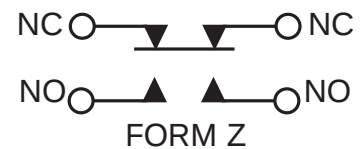
Circuit for microswitch version
