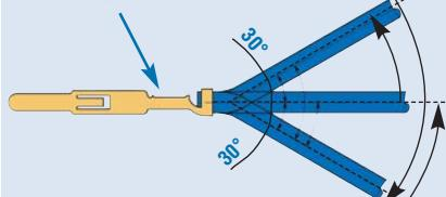
Insulation must be securely held after bend test
