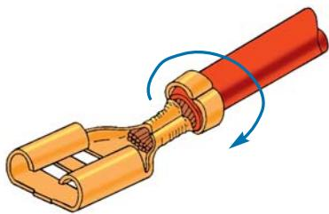
Cut off tab deformed
