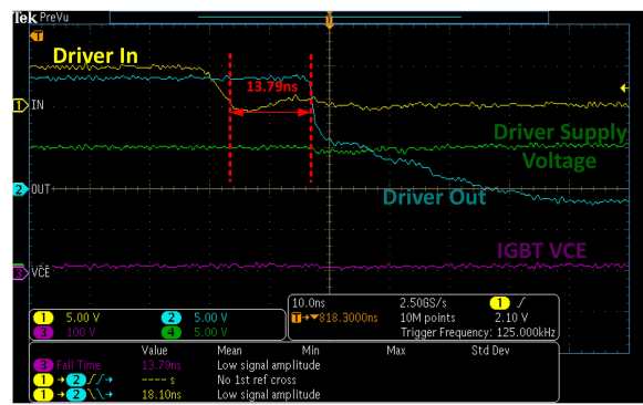
Figure 8-5. Turn-Off Propagation Delay Waveform
