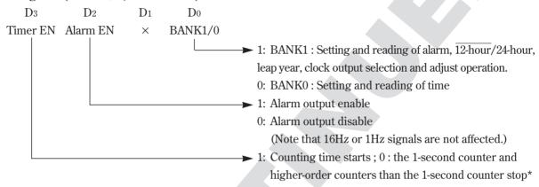
\*) When the Timer EN is set to 0, the 1-second counter and higher-order counters than the 1-second counter stop. If any carrying occurs in the lower-order counters than the 1-second counter while the Timer EN is 0, carrying will be held and avoided until the Timer EN changes from 0 to 1. Thus, no apparent delay is produced when the duration of the Timer EN = 0 is less than one second.
