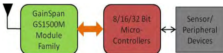
GS1500M based embedded Serial/IP to Wi-Fi application
