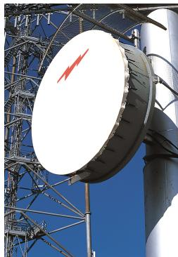
3.7 m | 12 ft High Performance Parabolic Shielded Antenna, single-polarized, 5.725–6.425 GHz, CPR137G, gray antenna, enhanced white radome with flash, standard pack—two-piece reflector
