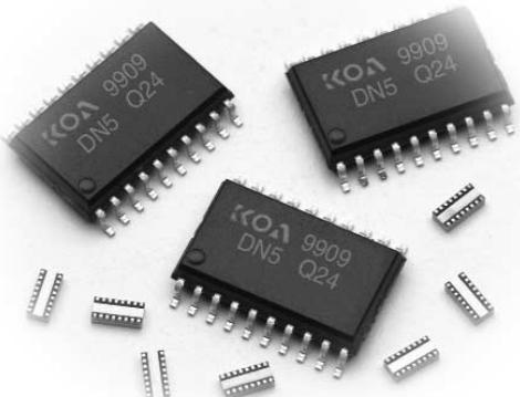
This diode network is designed to provide nineteen channels of active termination for high-speed data signals to eliminate signal undershoot and overshoot. The network has the added benefit of acting to suppress any ESD voltage events by shunting the energy to ground assuring maximum reliability of electronic systems in the field. Trigger levels are defined by the positive and negative bias levels set by the user.
