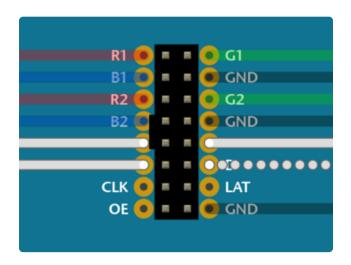
Pins A, B, C and D select which two rows of the display are currently lit. (32x16 matrices don't have a "D" pin — it's connected to ground instead.)
