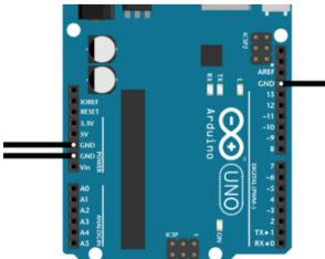
Arduino Mega boards have five ground pins. Same three as the Arduino Uno, plus two more next to pins 52 & 53.
