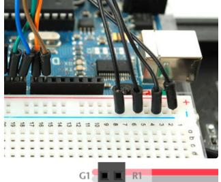
**32x32** and **64x32** matrices require **three** ground connections. **32x16** matrices have **four**.
