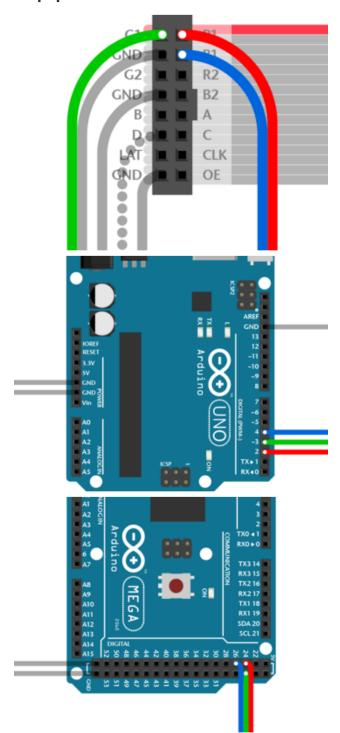
Pins **R1**, **G1** and **B1** (labeled R0, B0 and G0 on some matrices) deliver data to the **top** half of the display.
