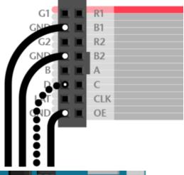
Current Arduino Uno form-factor boards have three ground pins (the third is next to pin 13). If you need additional ground connections — for a 32x16 matrix, or if using an older Arduino board with only 2 ground pins — a solderless breadboard is handy for linking all these pins.
