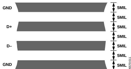
Figure 22. Typical Arrangement of Signal Tracks
