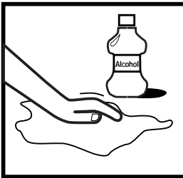
Clean surface with a clean cloth and isopropyl alcohol.
