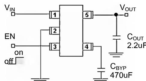
EN (Pin 3) may be connected directly to  $V_{IN}$  (Pin1)
