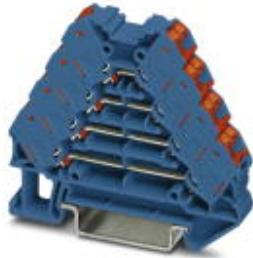
Marshalling panel, Nom. voltage: 250 V, Nominal current: 10 A, Cross section: 0.14 mm<sup>2</sup> - 2.5 mm<sup>2</sup>, AWG: 12 - 26, Connection type: Push-in connection, Width: 8.3 mm, Length: 64 mm, Color: blue, Assembly: NS 35/7,5, NS 35/15
