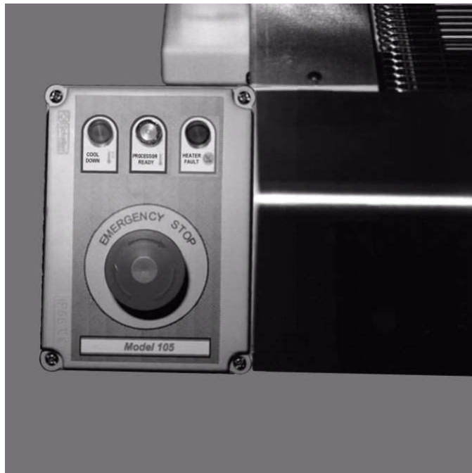
Emergency Stop Enclosure
