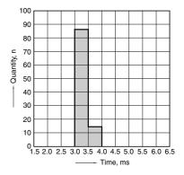
6. Distribution of release time Sample: CP1-12V, 100pcs Ambient temperature: 20°C 68°F
