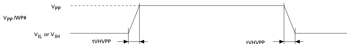
Figure 24: Accelerated Programming Timing Waveform
