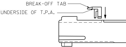
3. AFTER THE TERMINALS ARE LOADED INTO THE HOUSING, THE T.P.A. IS TO BE "BROKEN OFF". WITH THE BREAK-OFF TAB FACING FORWARD AS SHOWN, INSERT THE T.P.A. THRU THE HOLE IN TOP OF HOUSING UNTIL THE UNDERSIDE OF THE T.P.A. CONTACTS THE TOP SURFACE OF THE HOUSING. THIS RETAINS THE TERMINAL IN THE HOUSING UNTIL IT IS LOADED INTO THE SHROUD.
