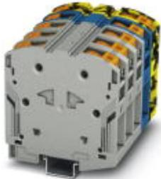
High-current terminal block, Blocked, Connection method: Push-in connection, Number of positions: 4, Cross section: 25 mm<sup>2</sup> - 95 mm<sup>2</sup>, AWG: 4 - 3/0, Width: 100 mm, Color: gray/black-yellow, Mounting type: NS 35/15
