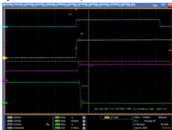
Figure 16: Turn ON output current characteristics (1)
