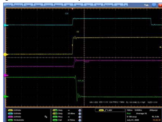
Figure 17: Turn OFF output current characteristics (2)
