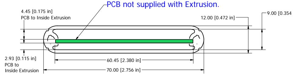
Extrusion designed for 60mm wide x 120mm long PCBs.
