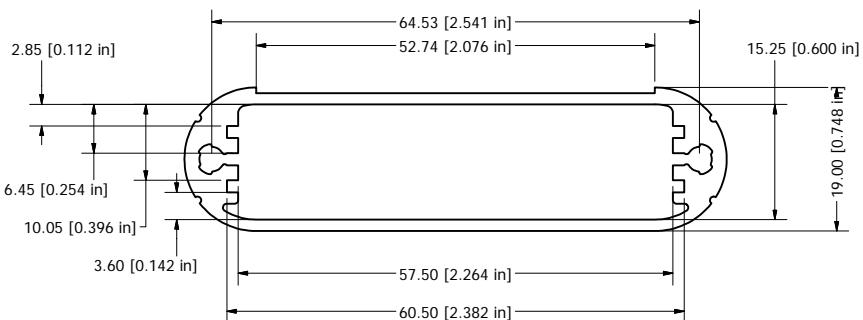
Extrusion designed for 60mm wide x 120mm long PCBs.
