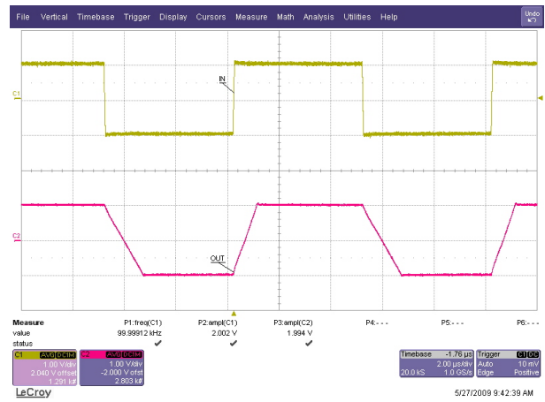
Figure 10. Non-Inverting Large Signal Step Response
