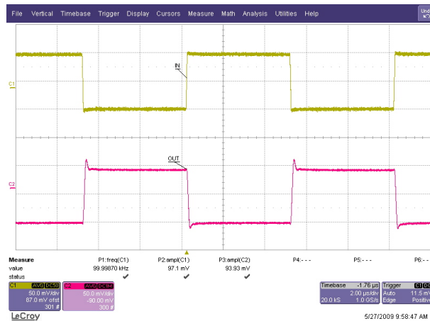
Figure 13. Inverting Small Signal Step Response
