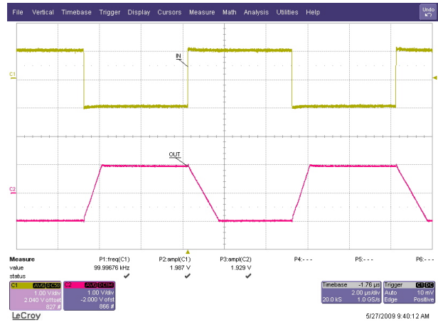
Figure 12. Inverting Large Signal Step Response
