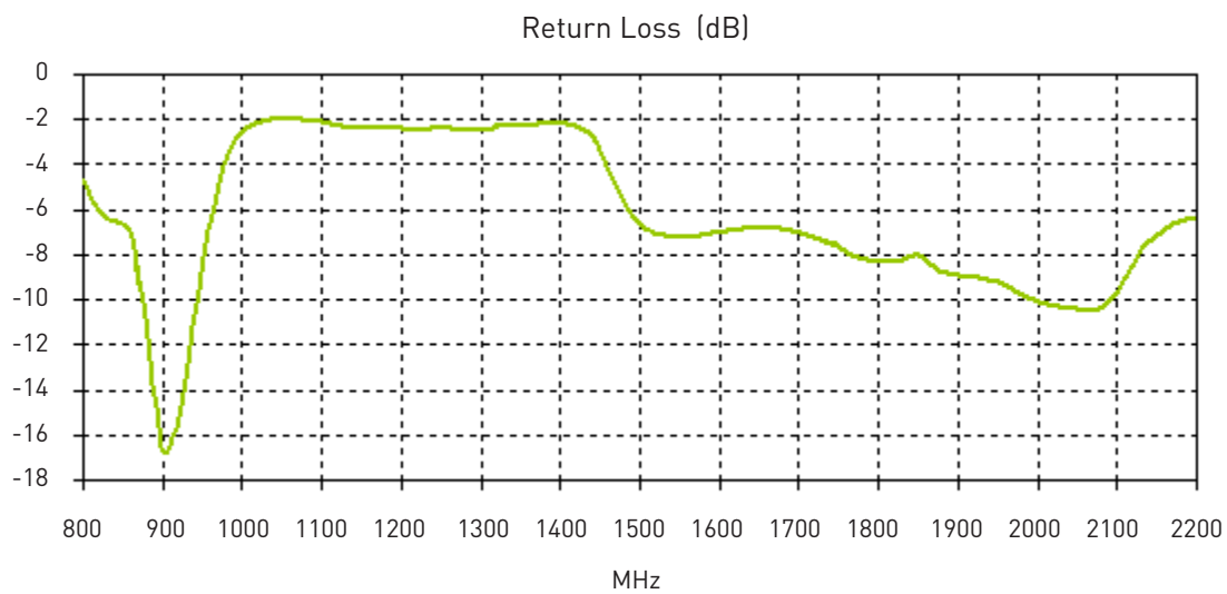
Figure 3. Return Loss for the FXP14 Antenna.
