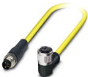
Sensor/actuator cable, 4-position, PVC, yellow, Plug straight M8, on Socket angled M12 SPEEDCON, A-coded, cable length: 0.5 m
