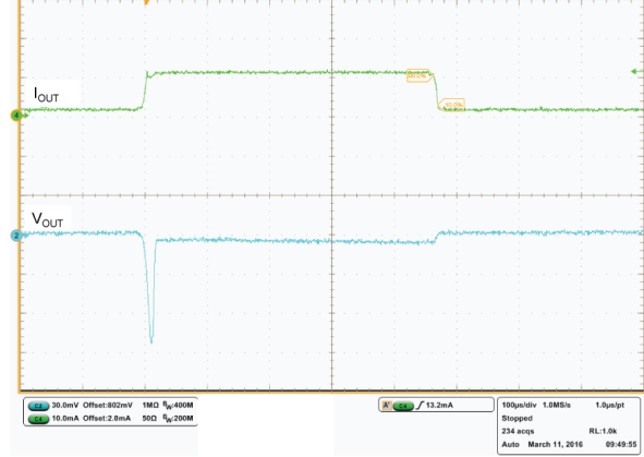
Figure 29. Load transient ( t_{rise} = 5 \mu s )
