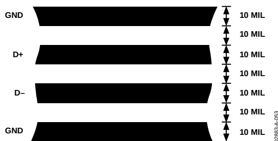
Figure 54. Arrangement of Signal Tracks
