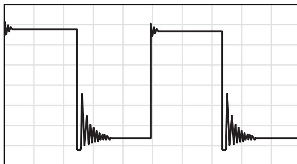
(b) C_L = 260 \text{ pF} , R_L = \text{NO LOAD}
