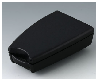
A9064109 SMART-CASE XS ABS (UL 94 HB) black RAL 9005 2.28"x1.40"x0.75" IP 40
