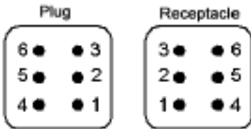
View from cable side
