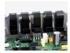
Bergquist Sil-Pad A1500 is a silicone-based, thermally conductive and electrically insulating material. It consists of a cured silicone elastomeric compound coated on both sides of a fiberglass reinforcement layer.
