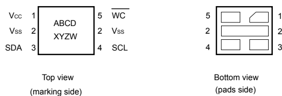
Figure 3. UFDFPN5 (DFN5) package connections
