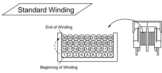
High-frequency noise can pass through the Filter easily because both edges of coils are close as shown above
