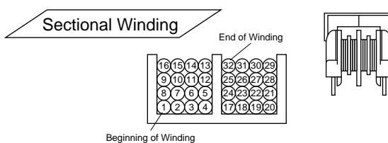
High-frequency noise can hardly pass through the Filter because both edges of coil are not close as shown above
