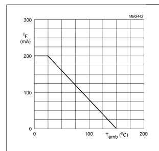
Device mounted on an FR4 printed-circuit board.
