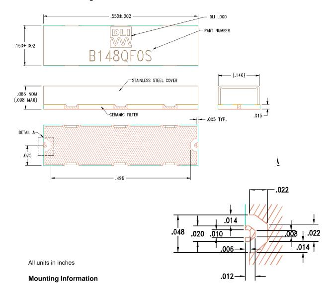
PCB ground pattern length and width can be 0.002-0.003 inches larger than filter footprint. Dimensions of filter launch and PCB launch pattern should be closely matched. It is suggested that PCB ground metal be pulled back from RF I/O trace to account for component alignment tolerance. Ground via depth and spacing should be set so as not to create any resonances at the frequency of operation.
