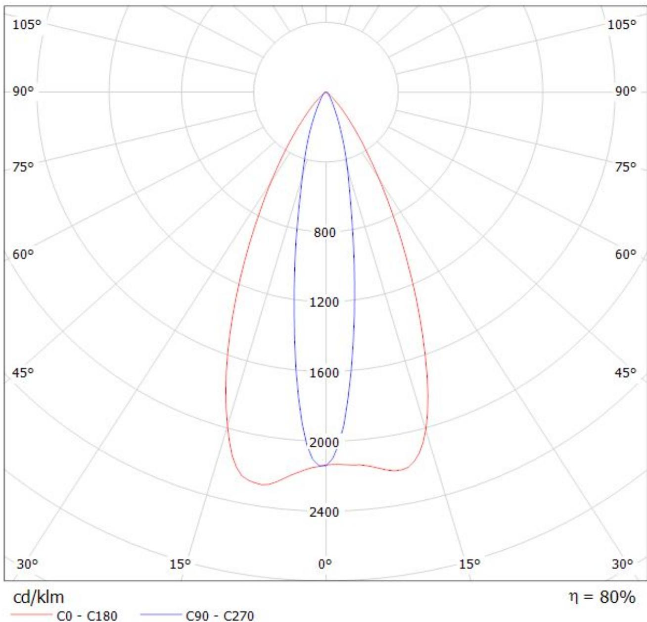
Luminaire: Ledil Oy FP11957 & FP11958\_LISA2-WWW (Osram Oslon 80 79lm @ 250mA) Efficiency=74%
