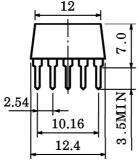
Unit in mm Tolerance is  $\pm 0.25$ Unless otherwise noted.
