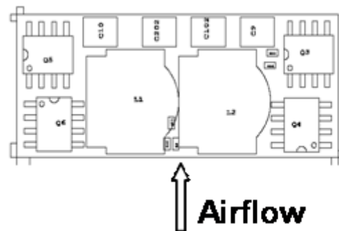
Figure 34. Airflow direction for thermal testing.
