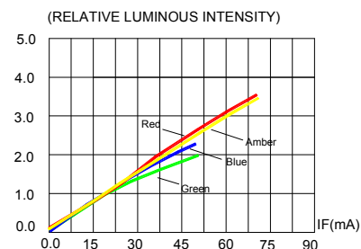
FIG.2 RELATIVE LUMINOUS INTENSITY VS. FORWARD CURRENT
