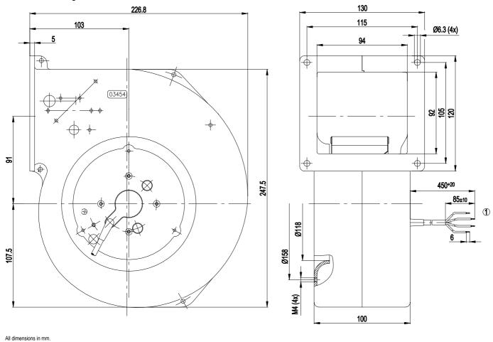
Cable PVC 4G 0.5 mm<sup>2</sup>, 4x crimped splices
