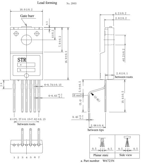
Pin material: Cu Pin treatment: Ni plating and solder dip Product weight (approximate): 2.3g
