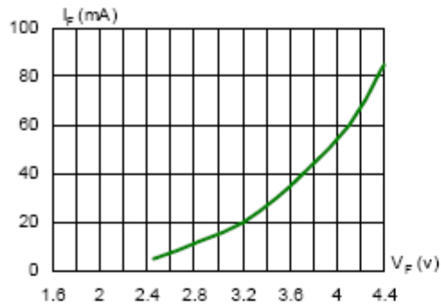
Fig.1 Forward Current vs. Forward Voltage
