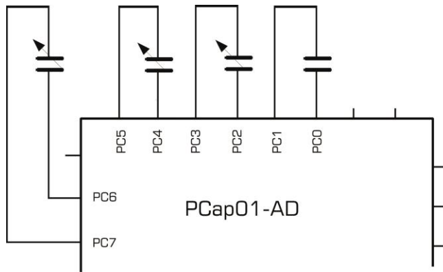
Figure 3-6: Single sensors, floating, up to 3 sensors (C1 to C3) and one reference (C0)
