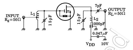
L<sub>1</sub>: 1.0 mmφ silver plated copper wire 4.0 T, 8 mmφ ID TAP at 1.0 T from coil end
