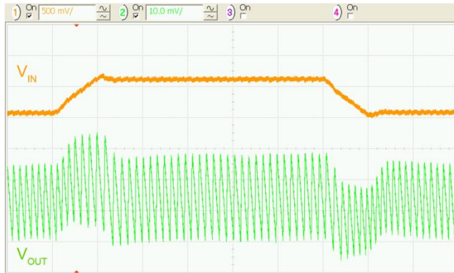
Figure 20. Line Transient 3.3 V_{IN} to 3.9 V_{IN} , 50 mA Load, 10 \mu\text{s/div.}
