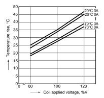
3-(2). Coil temperature rise Sample: ALA2PF12, 6 pcs. Measured portion: coil inside Contact current: 0 A, 5A
