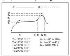
Temperature rise of relay itself may vary according to the mounting level or the heating method of reflow equipment. Therefore, please set the temperature of soldering portion of relay terminal and the top surface of the relay case not to exceed the above mentioned soldering condition.
