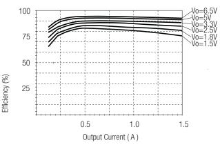
Efficiency Vs Load (Vin=Max)
