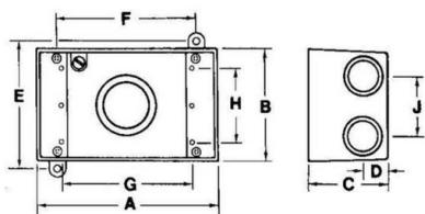
Alloy A380 aluminum, certified zinc alloy and stainless steel springs provide increased corrosion resistance
