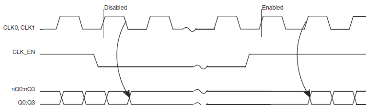
FIGURE 1. CLK_EN TIMING DIAGRAM
