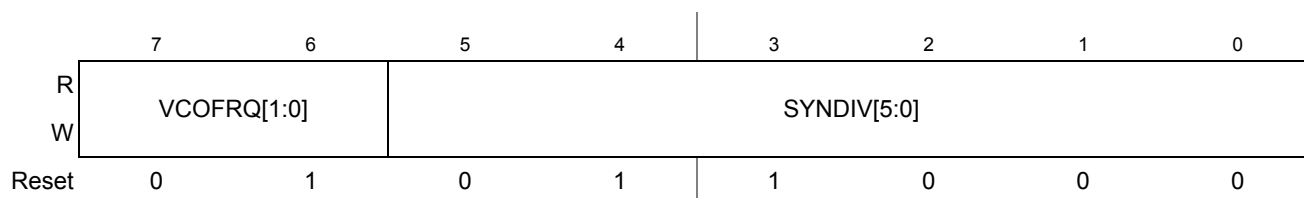
Figure 9-7. S12CPMU_UHV Synthesizer Register (CPMUSYNR)
