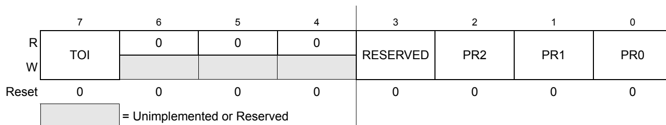
Figure 16-15. Timer System Control Register 2 (TSCR2)
