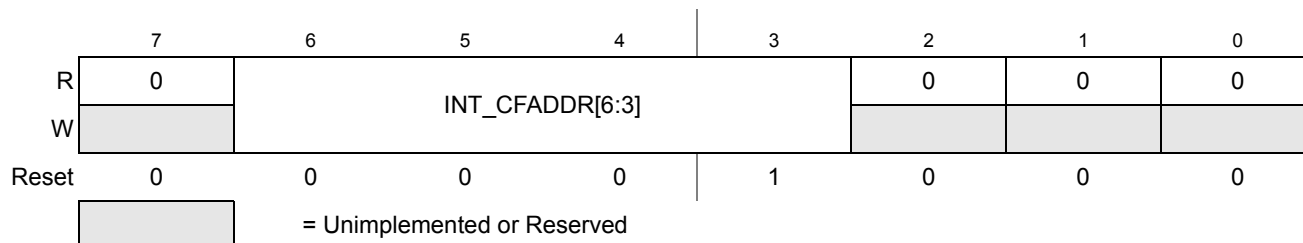
Figure 6-4. Interrupt Configuration Address Register (INT_CFADDR)
