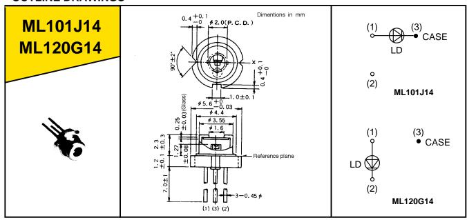
There is no model with a monitor photo diode in ML1XX14 series.
